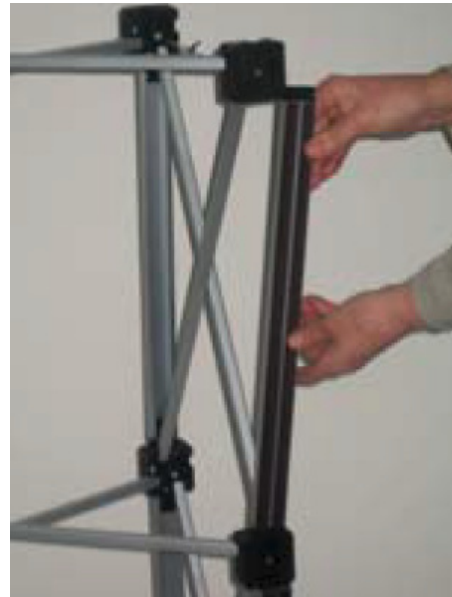
Push together to make hooks catch
