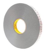
A thick grey double coated acrylic foam tape with paper liner. The multi-purpose acrylic adhesive on both sides bonds to a broad range of high and medium surface energy substrates including metals, glass and a wide variety of paints and plastics as well as plasticised vinyl. The conformable foam provides good contact between substrates even when they are slightly mismatched.
