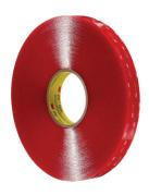
A thick clear double coated acrylic foam tape with PE film liner. The general purpose acrylic adhesive on both sides bonds to a broad range of high surface energy substrates including metals, glass and easier to bond paints and plastics. The clear tape is good for bonding transparent or translucent materials or for applications where colourless is a benefit.
