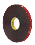
A thick black double coated acrylic foam tape with PE film liner. The modified acrylic adhesive on both sides bonds to a broad range of high, medium and medium/low surface energy substrates including metals, glass and a wide variety of plastics and paints, including many powder coated paints. The very conformable foam provides good contact between substrates even when they are slightly mismatched.
