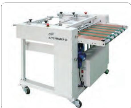
Automatic aligning & stacking device for perfect alignment.
