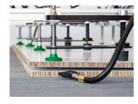
Additional separating unit (rear) for reliable separation of panel material, consisting of four bellows suction units and two separating nozzles:
